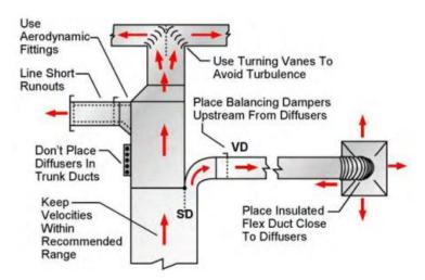
Figure 35: Options for Decreasing Noise in Ductwork, Carrier
