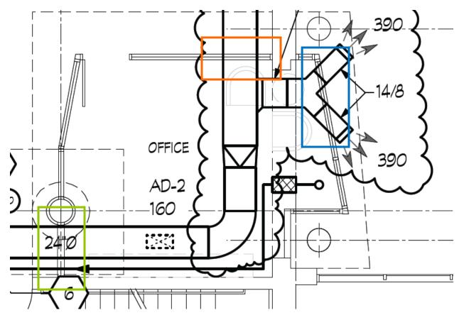
Figure 37: Duct Penetrations through Glass Curtain wall, SvS Architectural Drawings
