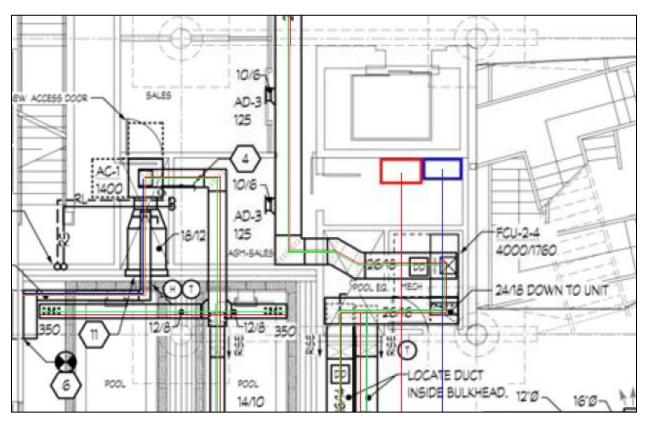
Figure 33: Proposed Supply and Exhaust Duct Location
