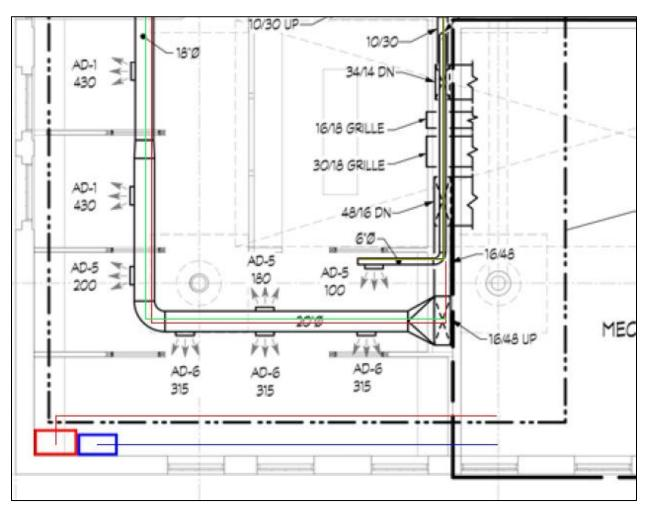
Figure 32: Proposed Supply and Exhaust Duct Location
