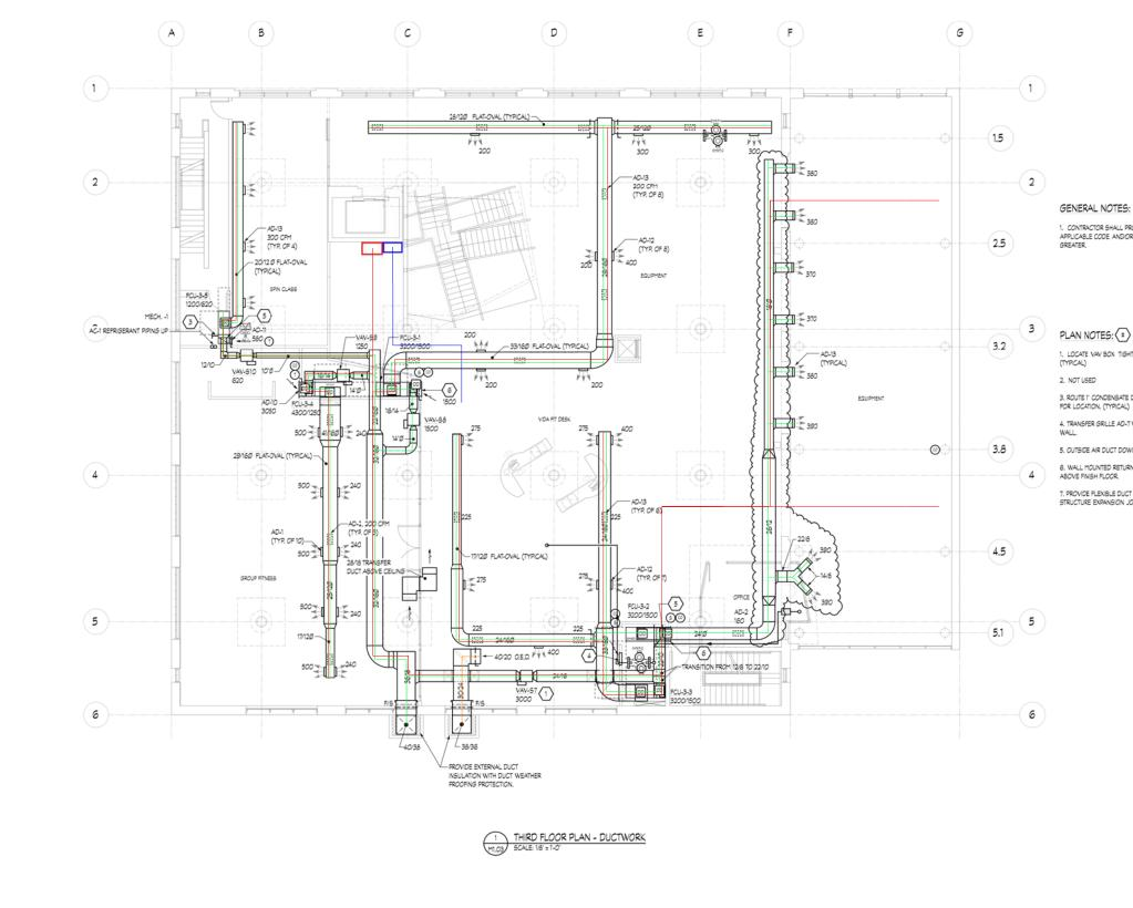
1. CONTRACTOR SHALL PROVIDE EQUIPMENT WITH REQUIRED CLEARANCES PER APPLICABLE CODE AND/OR MANUFACTURE'S RECOMMENDATION WHICHEVER IS GREATER.
