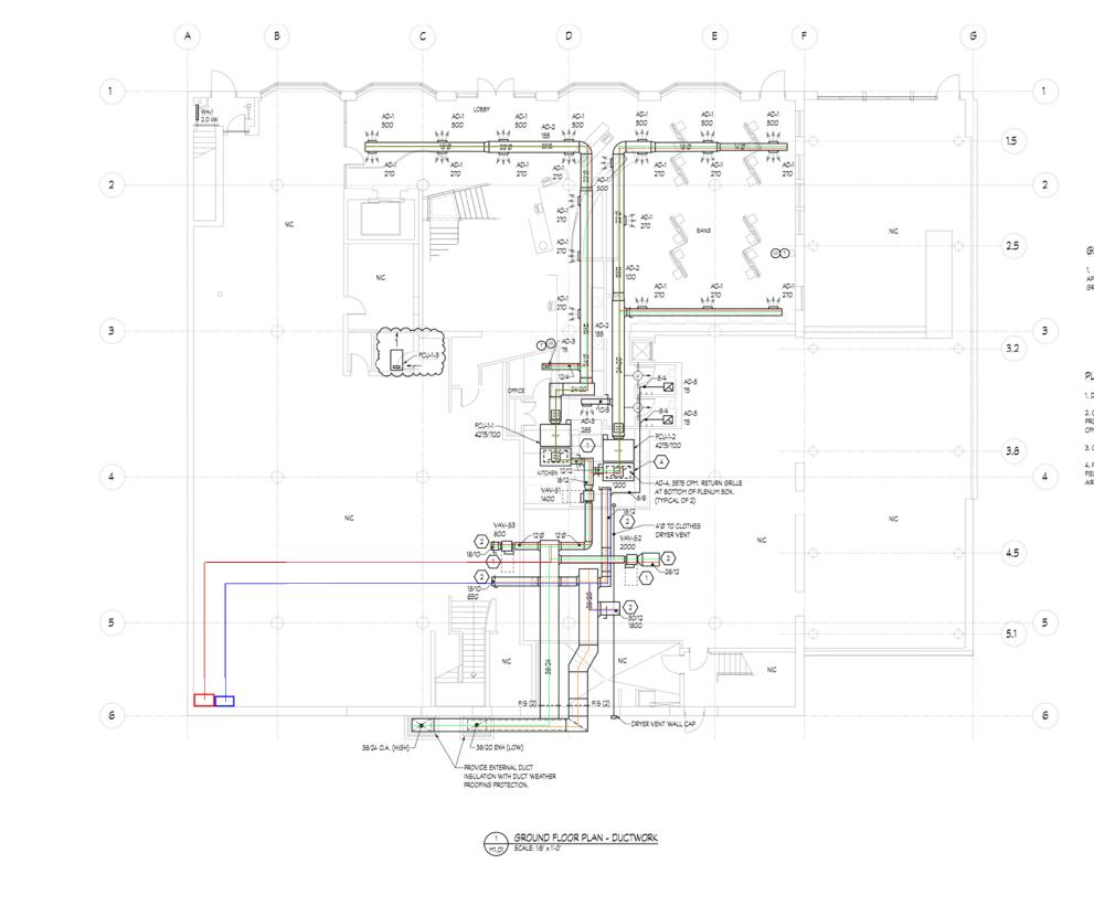
3. CONNECT TO EXISTING BASE BUILDING MEDIUM PRESSURE DUCT. 4. PROVIDE WITH PLENUM BOX WITH FLLL SIZE EQUAL TO UNIT INLET, FIELD COORDINATE PLENUM BOX DEPTH TO FIT RETURN AND OUTSIDE AIR DUCTWORK. (TYPICAL)
